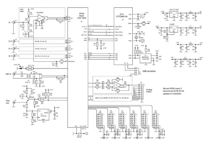
**Core device**: The core element is an Mach XO2 FPGA with 2000 or more gate blocks. The default desgin works with a XO2-2000HC-6 device. It features 48 digital output lines grouped in 6 blocks of 8 bits, which can be connected to an 9-fold NIM output board, or an 8-fold TTL output board. (to be documented).
