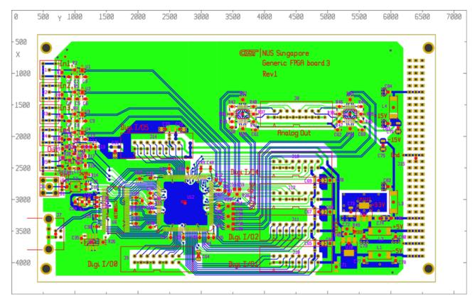
The component-side inner layer is for ground only, the bottom-side inner layer carries mostly a +3.3V supply.
